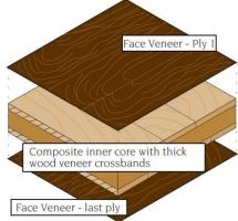
Medium Density Fiberboard Core Plywood
