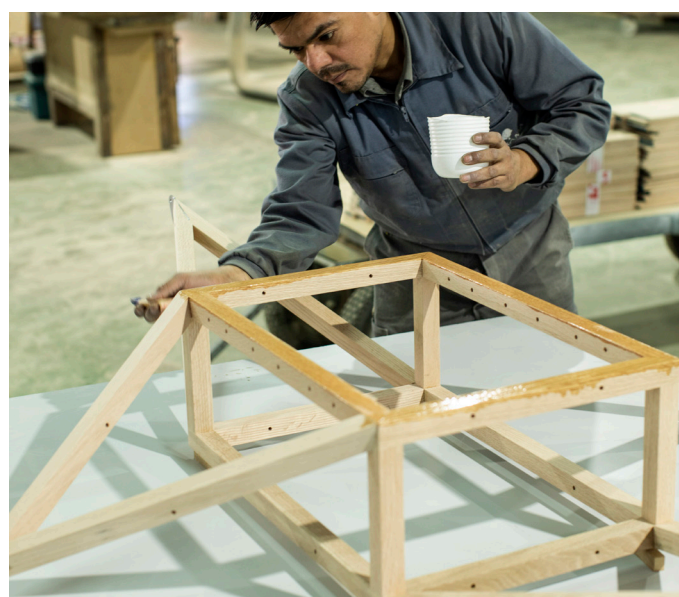
American red oak frames, part of the Venice Biennale project with EMBT, being oiled in Spain.
